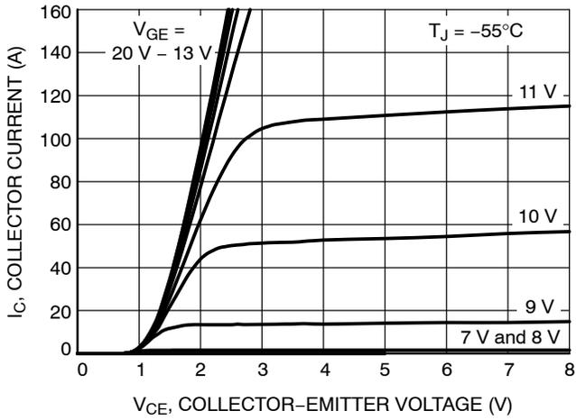
Figure 3. Output Characteristics
