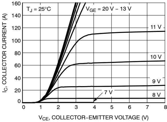
Figure 1. Output Characteristics
