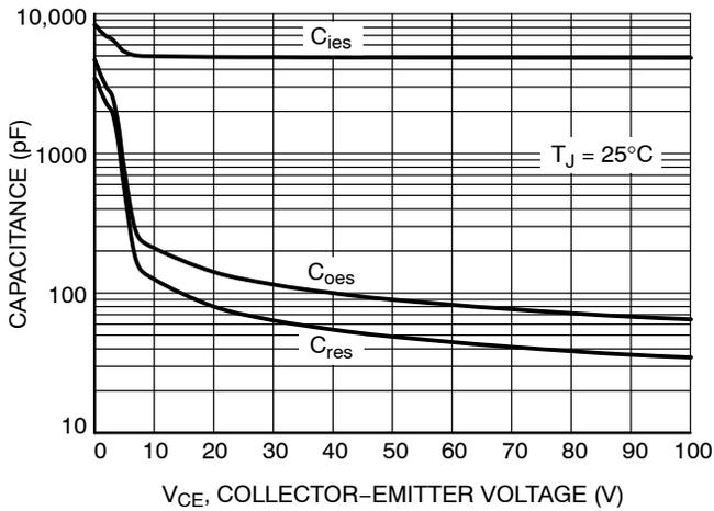
Figure 7. Typical Capacitance
