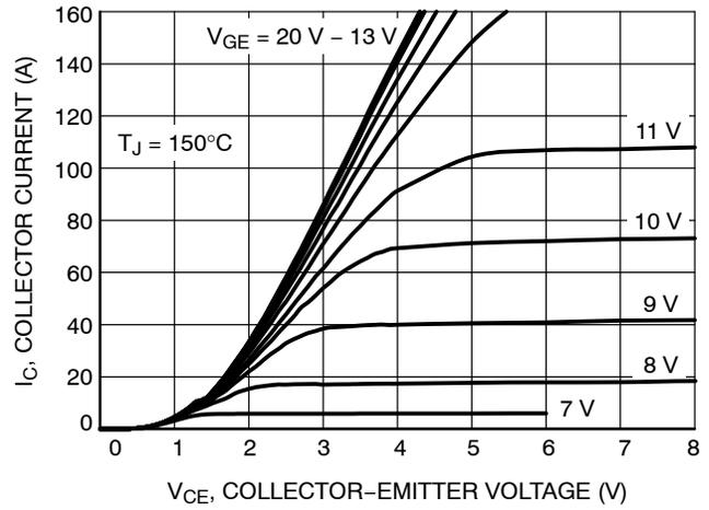
Figure 2. Output Characteristics
