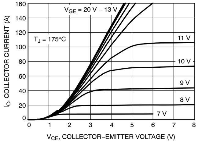
Figure 4. Output Characteristics
