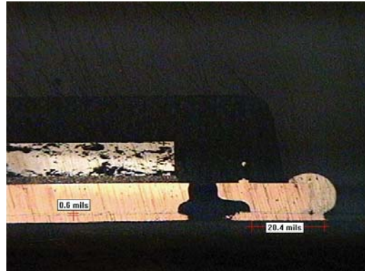
37% Paste coverage, Encroached Via, 0.6 mil Standoff
