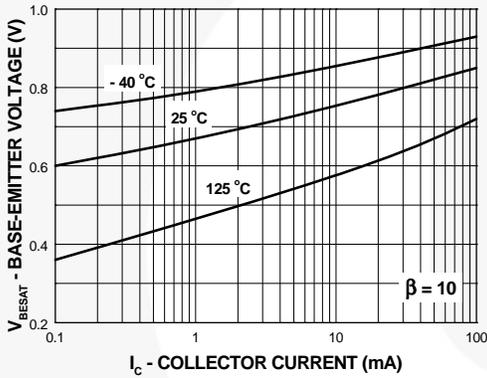
Figure 3. Base-Emitter Saturation Voltage vs. Collector Current
