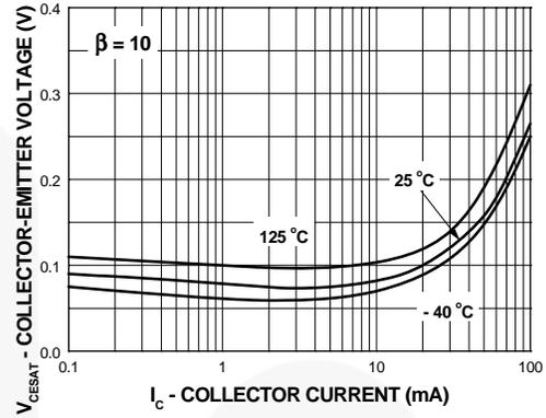
Figure 2. Collector-Emitter Saturation Voltage vs. Collector Current
