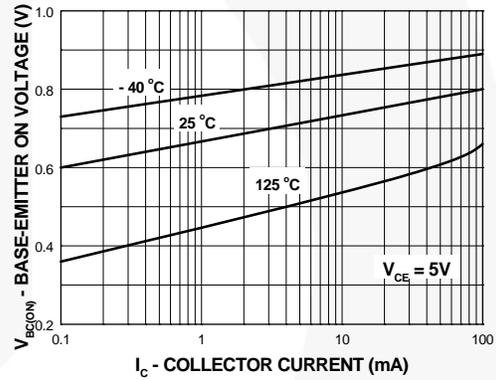
Figure 4. Base-Emitter On Voltage vs. Collector Current
