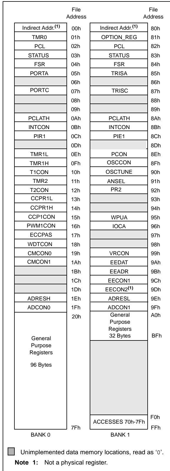
FIGURE 2-2: DATA MEMORY MAP OF THE PIC16F684
