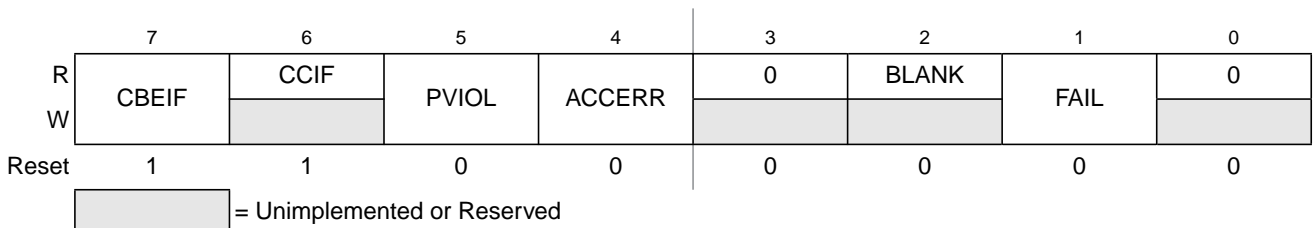
Figure 26-10. EEPROM Status Register (ESTAT — Special Mode)
