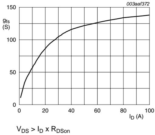
**Fig 11. Forward transconductance as a function of drain current; typical values**
