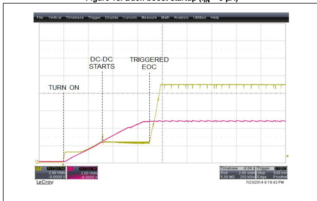
Figure 13. Buck-boost startup ( I_{IN} = 5 \mu A )
