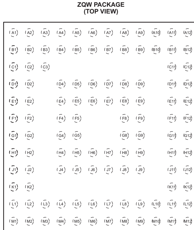
Figure 4-3. 113-Pin ZQW Package (Top View) – MSP430F5338, MSP430F5336, MSP430F5335, MSP430F5333
